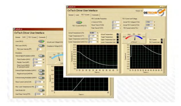
Users have full control of the fiber coupled laser module power through a PC controlled digital interface. The units are supplied with RS232 I/O and LabView drivers. They can also be ordered with a USB interface adapter. Laser output power is set by adjusting the current level (ACC mode) or adjusting the laser in automatic power (APC) control mode. The APC mode utilizes the laser diode's internal monitor photo-diode to feedback to the bias current and temperature controller.
