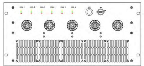
Device dimensions: 19" (483mm), 5HU (221.5mm), 340mm depth excluding front and rear handles
