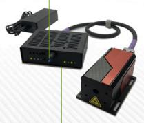
Pre-set current limit & temperature limits keep laser diode in safe operating range; ESD & surge clamps protect laser diode from all power surges
