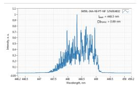
Typical spectrum of 0450 nm diode laser. Measured with 10 pm resolution.
