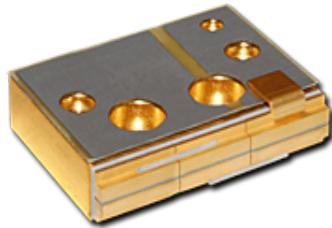
The AAA package is a compact, conductively-cooled laser diode array. The AAA package is available in pulsed configurations with up to 7.2 kW of peak power or in CW configurations with up to 120 W of continuous power.
