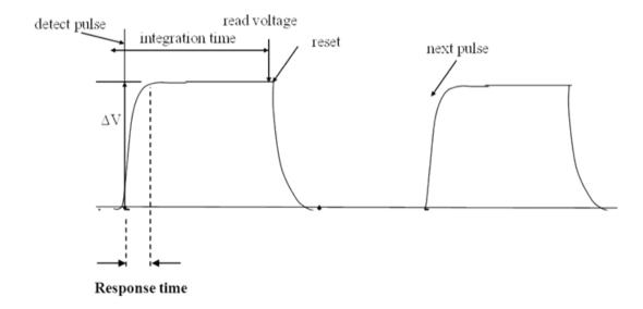
When the user sets the "maximum pulse width," for example  $2\mu s$ , this sets the integration time. Even if the pulse width is actually only 3ns, the sensor will hold the voltage for  $2\mu s$  (in this example) and "integrate it," i.e. collect and measure it.
