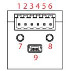
The high speed modulation option does not include the coaxial modulation inputs (7 and 8) and the digital low-speed modulation input (5) on the controller. Instead, a high speed digital modulation input (MMCX) is placed directly on the back of the laser head.
