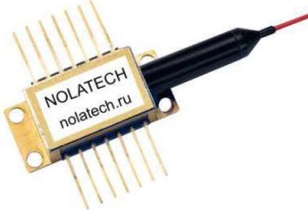
FPL-FBG-1550-14BF-150 is FBG-stabilized laser diode module designed for optical measurement and communication. The laser is packaged in 14-pin standard butterfly package with monitor photodiode and thermo-electric cooler (TEC). Module is pigtailed with 0,7-1,0 m of single mode polarization maintaining fiber and connectorized by FC/APC connector.
