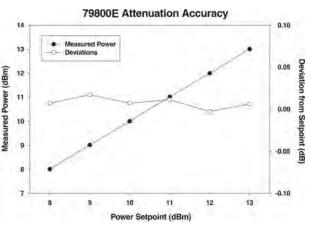
Industry-leading fiber optic source power attenuation accuracy.
