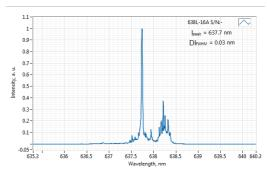
Typical spectrum of 0638 nm diode laser. Measured with 20 pm resolution.
