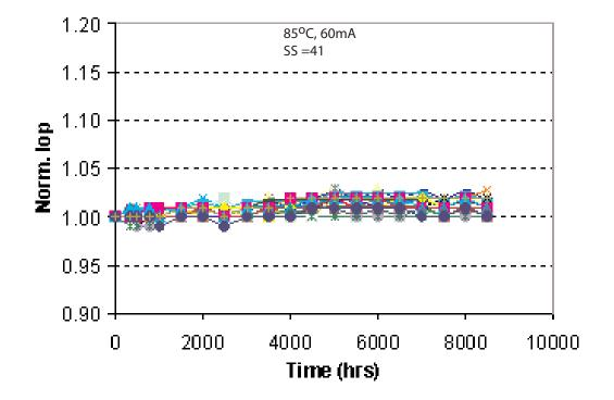
Normalized operating current at 5mW, 25C after aging at 85C
