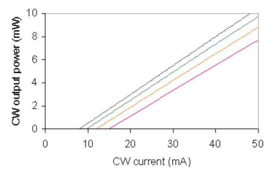
Typical IV curve at  $T_{C}=25^{\circ}C$ ,  $45^{\circ}C$ ,  $65^{\circ}C$  and  $85^{\circ}C$
