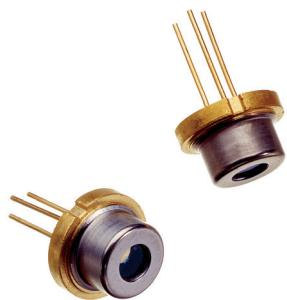
The Intense-HPD Series 4000 diode lasers are single mode, index guided quantum well structures. The lasers provide high power, low astigmatism, and narrow spectral width with a single spatial mode Gaussian far field.
