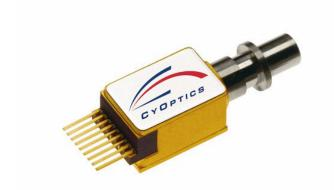
CyOptics' 1610 and 1611 type TOSA is available with LC receptacle (for use in DWDM SFP and other pluggable transceivers) or fiber pigtail (for use on line cards)
