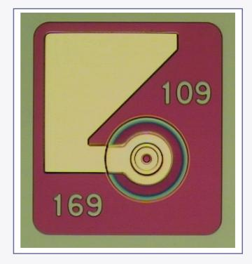
Oclaro's single mode VCSELs are designed to meet stringent specifications for a broad range of optical sensing applications. This product offers polarization stable single mode emission with a symmetrical Gaussian beam profile and output powers of typically 1mW. Bias currents range from 3 to 6mA.
