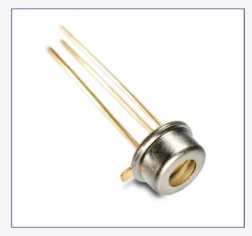
Oclaro's single mode VCSELs are designed to meet stringent specifications for a broad range of optical sensing applications. This product offers polarization stable single mode emission with a symmetrical Gaussian beam profile and output powers of typically 1mW. Bias currents range from 3 to 6mA.
