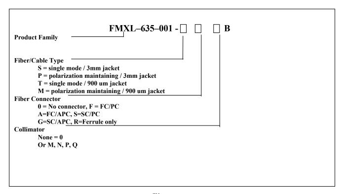
Example: FMXL-0635-001-SF0B, FiberMAX635<sup>TM</sup> laser module with 635nm Laser diode, 1.8mW power output, single mode fiber in 3mm jacketing, FC/PC connector, no collimated beam output optics, B pinout.
