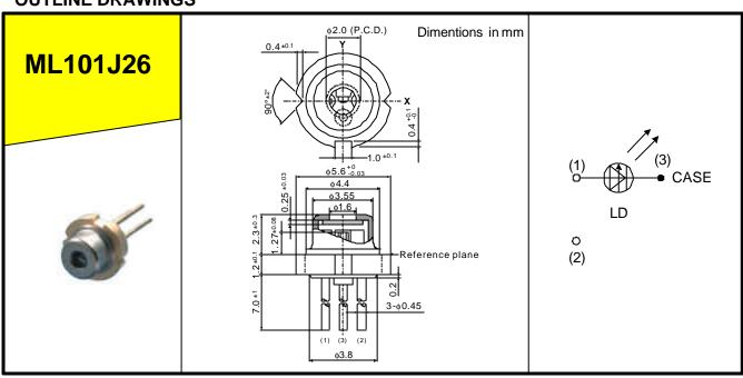
There is no model with a monitor photo diode in ML1XX26 series.
