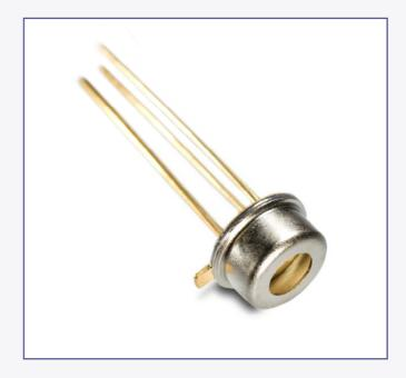
Oclaro's 760nm VCSELs are designed to meet the requirements for the optical measurement of oxygen concentration levels as well as other spectroscopic applications. The laser emits a single transverse and longitudinal mode with stable linear polarization, small divergence and a highly symmetrical Gaussian beam shape. The VCSEL is assembled in a hermetic TO46 package with flat AR coated glass window.
