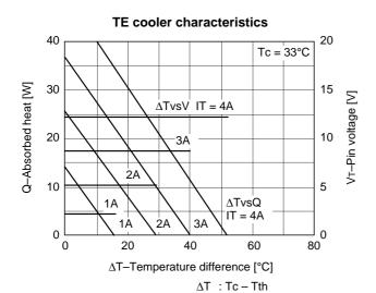
Tth: Thermistor temperature Tc : Case temperature
