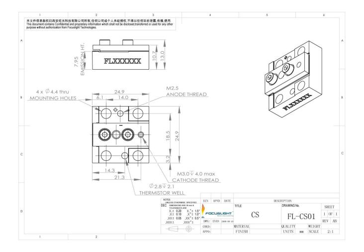
This structure drawing is only for reference. More structure drawings can be found below the datasheet. For any other special requirement, please feel free to contact us.
