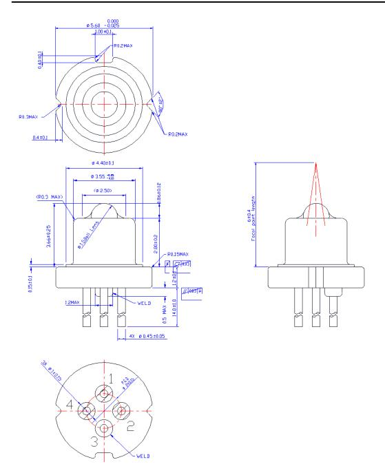
1.5 mm Ball Lens Type B (focal length =  $6.0 \pm 0.4$  mm)
