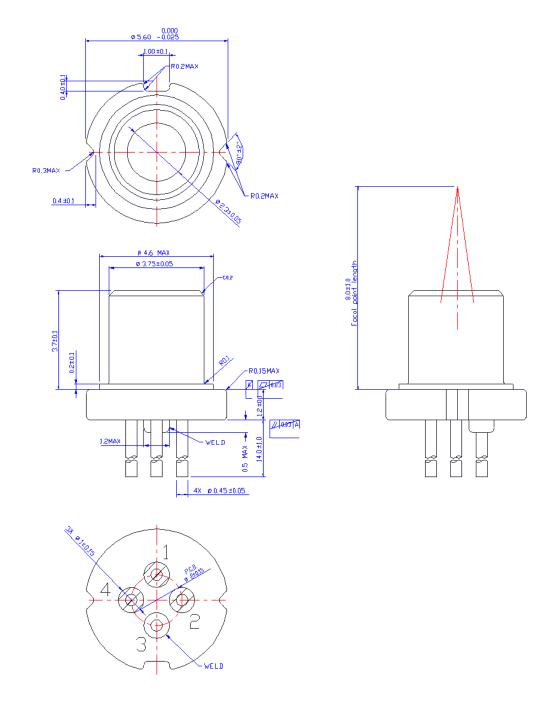
Aspherical Lens type A (focal length =  $8.0 \pm 1.0 \text{ mm}$ )
