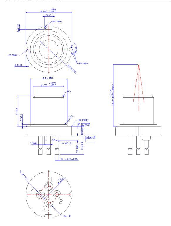
Aspherical Lens type A7 (focal length =  $7.5 \pm 1.0 \text{ mm}$ )
