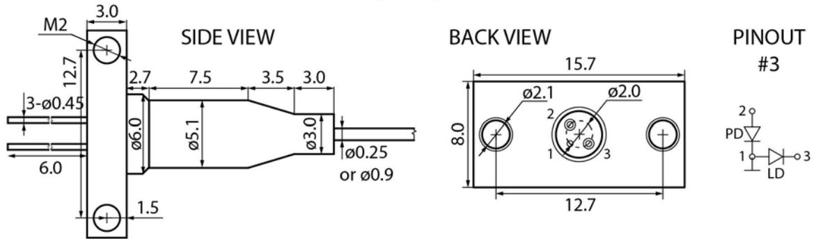
Connector FC/UPC, FC/APC, no connector, or by request
