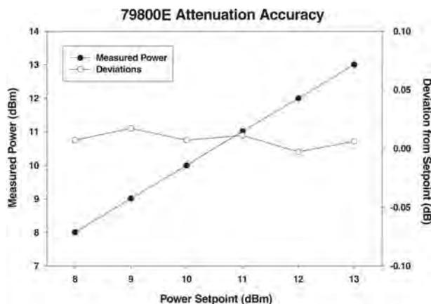
*Industry-leading fiber optic source power attenuation accuracy.*
