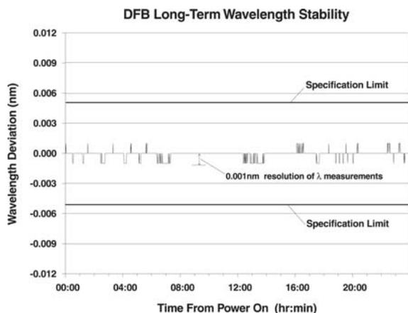
*Precise control of laser diode temperature and current densities ensures a stable wavelength.*
