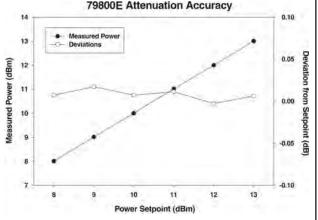
Industry-leading fiber optic source power attenuation accuracy.
