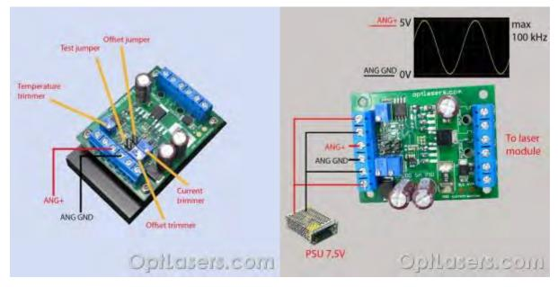
Recommended supply voltage is 7.5V. Higher voltage can lead to overheating of the driver. Nevertheless, power supply up to 12V may be used. Before turning on the power supply, make sure that all cables are connected correctly.
