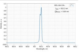
Typical spectrum of 0915 nm diode laser. Measured with 20 pm resolution.
