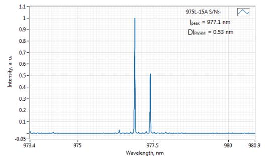
Typical spectrum of 0975 nm diode laser. Measured with 20 pm resolution.
