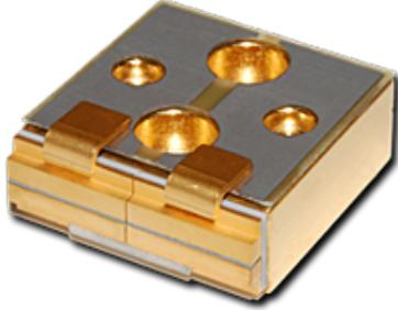
The AA package is a compact, conductively-cooled laser diode array. The AA package is available in pulsed configurations with up to 4.8 kW of peak power or in CW configurations with up to 80 W of continuous power.
