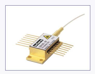
The Oclaro LC96A10xx-20R high power laser module has been designed as a light source for pulsed fiber lasers and CW applications that require 10xx nm single mode light. Processes and techniques of coupling the fiber to the laser allow high output powers that are very stable with both time and temperature. Devices are available with kink free output powers to 400mW CW.
