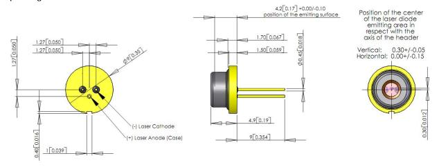
The 9 mm laser TO-can package is a widely accepted industry standard well-suited for low-power laser applications. However, the maximum output power is typically limited by the poor heat dissipation properties of the 9 mm package itself. Please contact us to discuss the best package option for your application.
