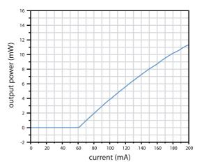
Fig. 2 Output power versus current characteristics of a 2700 nm FP laser diode at room temperature
