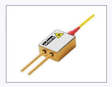
The Oclaro BMU4-808-02-R01/R02 multimode laser diode module series has been designed to provide the high power and reliability required for pumping solid-state lasers and for direct applications. The module includes a multimode laser diode chip with E2 front mirror passivation that prevents Catastrophic Optical Damage (COD) to the laser diode facet even at very high power levels. The coupling process allows for high output powers that are very stable with both time and temperature.
